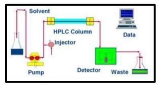
Figure 1: Flow Diagram of HPLC
