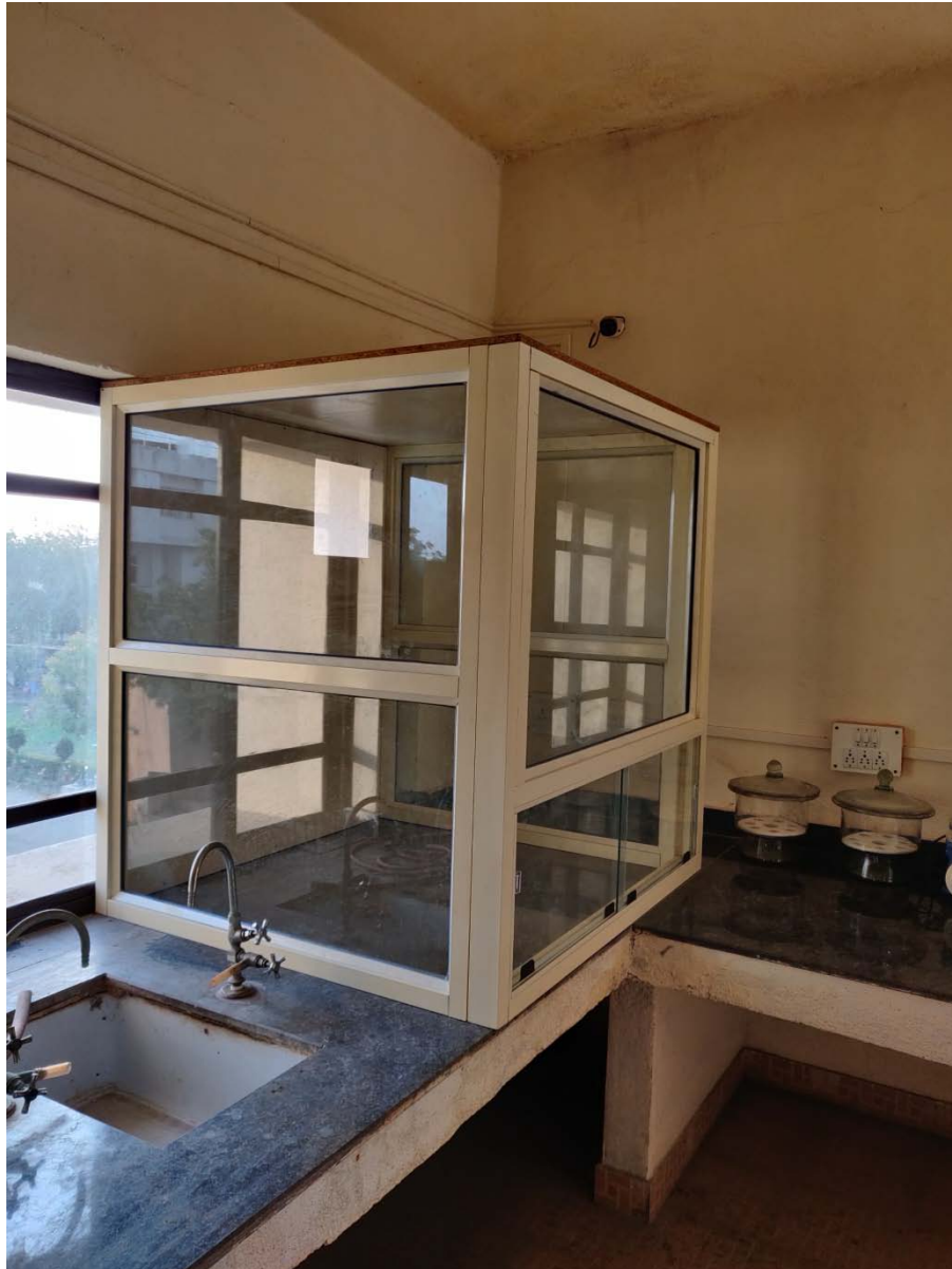
Fuming Cup Board for hazardous chemicals
